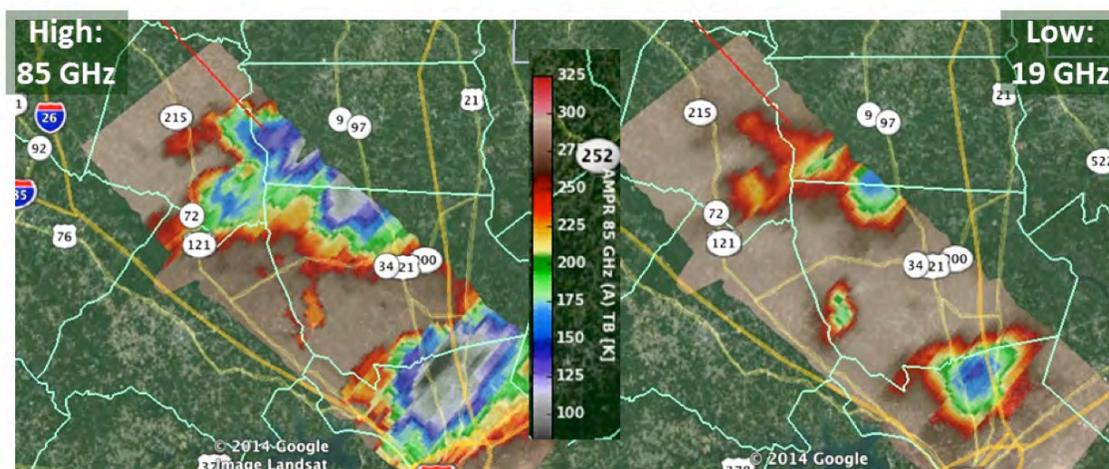
**Figure 5.** *Microwave brightness temperatures during severe storm convection.* These data—at high frequency [left] and low frequency [right]—in severe convection were observed by the AMPR radiometer aboard the ER-2 during a GPM Core satellite overpass at approximately 2316 UTC on May 23, 2014. Regions of increasing intensity are shown as nominally concentric color changes. **Image credit:** NASA
